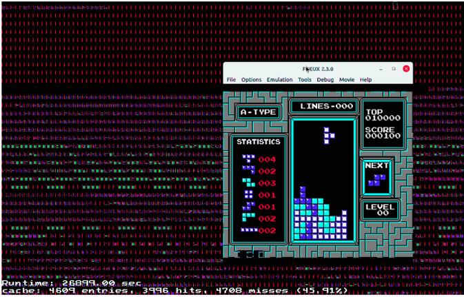
Figure 10: Playing a game of Tetris in the FCEUX emulator, in which we loaded the `tetris.nes` ROM from the `tetru` drive. The backdrop is a truncated portion of the visualization showing the contents of the 8,640 Tetris boards being emulated. The upper portion is the FAT-12 header and directory entries (it is mostly `0x00`) and the lower portion is the ROM data. I only have 100 points right now but as you can see I am gearing up to complete some sweet, high-scoring Tetrises.
