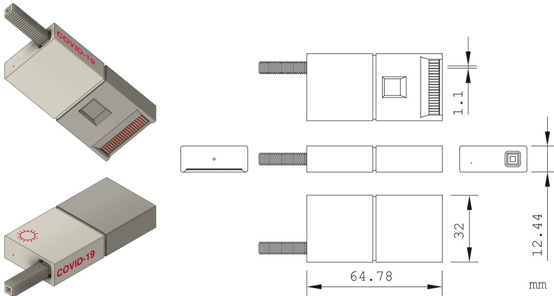
Figure 12: Mechanical drawing of the Cue COVID-19 test cartridge. The protruding stick is the nasal swab, which is permanently captured during use with zip-tie-like ratcheting. The card edge connector is the low tolerance piece here, whose small size (0.05 inch pitch with 1.1mm fingers) requires special consideration for mounting and soldering. (In its normal usage, this connector mates with some spring-loaded pins when the cartridge is inserted in the Cue reader.)
